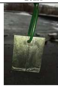
Zinc coated iron plate with worn out surface
