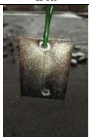
Chrome coated iron plate with worn out surface
